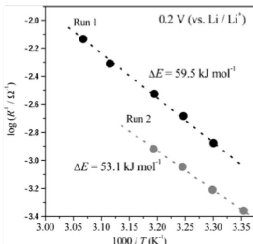
Temperature-dependence of  $R_{\text{ct}}$  @0.2 V vs. Li/Li<sup>+</sup>
