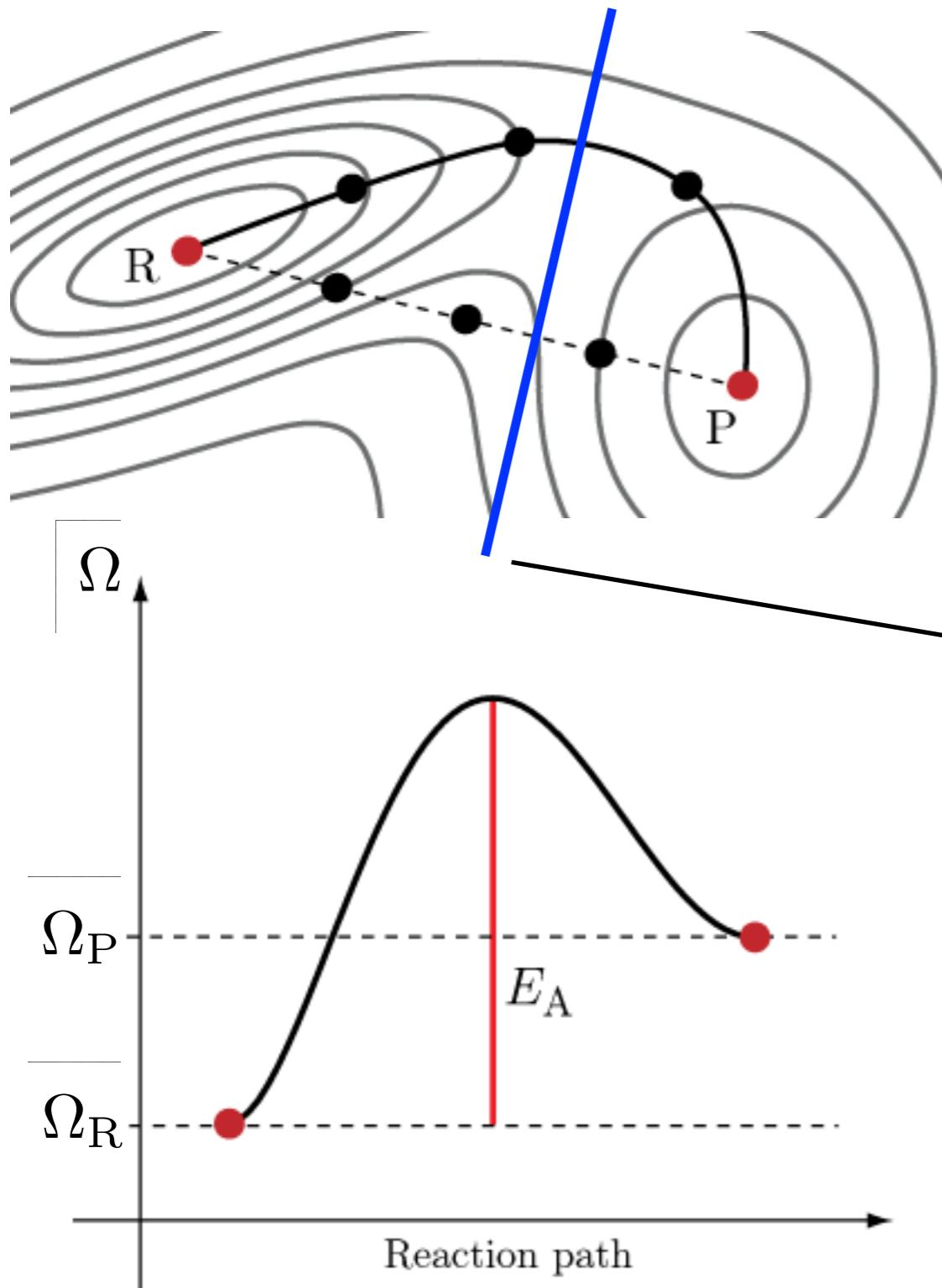
Searching the minimum energy path (MEP) using NEB with constant- $\mu$
